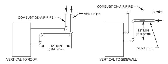
NOTE: A 12-in. (304.8mm) minimum offset pipe section is recommended with short (5 to 8 ft / 1.5 to 2.5M) vent systems. This recommendation is to reduce excessive condensate droplets.
